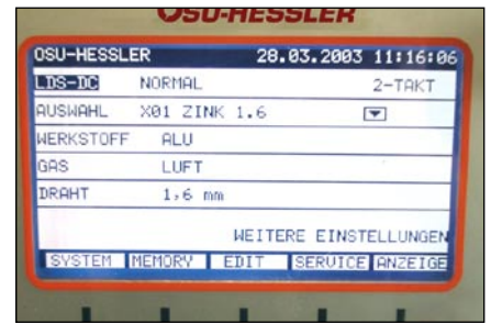
A big clearly arranged LCD-Display shows all necessary spray parameters and settings
